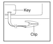
console to be ready for use. IMPORTANT: In an emergency, the key can be pulled from the console, causing the walking belt to slow to a stop. Test the clip by carefully taking a few steps backward; if the key is not pulled from the console, adjust the position of the clip.
